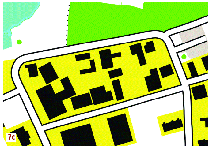
Figures 7a–7c. A Laser-Scan "mesoagent" generalizes the original cluster of buildings (a) to remove extraneous detail (b), then combines sub-groups of the cluster for clarity of display at a smaller scale (c).
