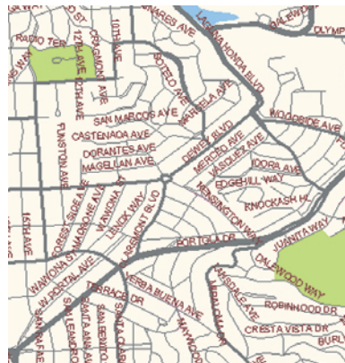
FIGURE 2 At 1:35,000 scale, the 5-point Arial street name labels still fit onto this Tele Atlas (www.teleatlas.com) basemap of San Francisco.
