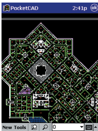
FIGURE 4 PocketCAD displays CAD architectural plan data of an office layout on a Compaq iPAQ.
