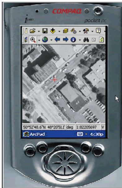
FIGURE 1 A 0.5-foot resolution orthophoto shown at 1:1,200 scale in ESRI's ArcPad on a Compaq iPAQ.
