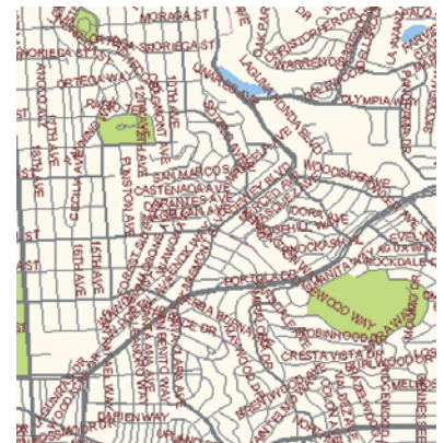
FIGURE 3 At 1:50,000 scale, the same 5-point Arial labels obscure each other or underlying street lines.
